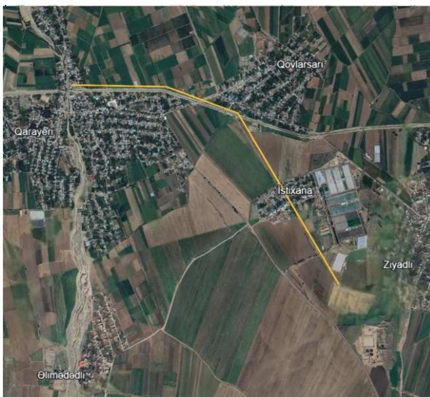
Figure 3. Proposed effluent discharge pipeline route from Ganja WWTP to irrigation canal and river 12
